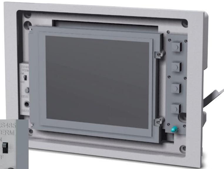
The front bezel can be removed for programming and touchscreen resetting, and to adjust the termination switch without the need to remove the unit from the wall. Optional bezels in Black, Ivory, White or Almond may be purchased separately to replace the standard white bezel.
